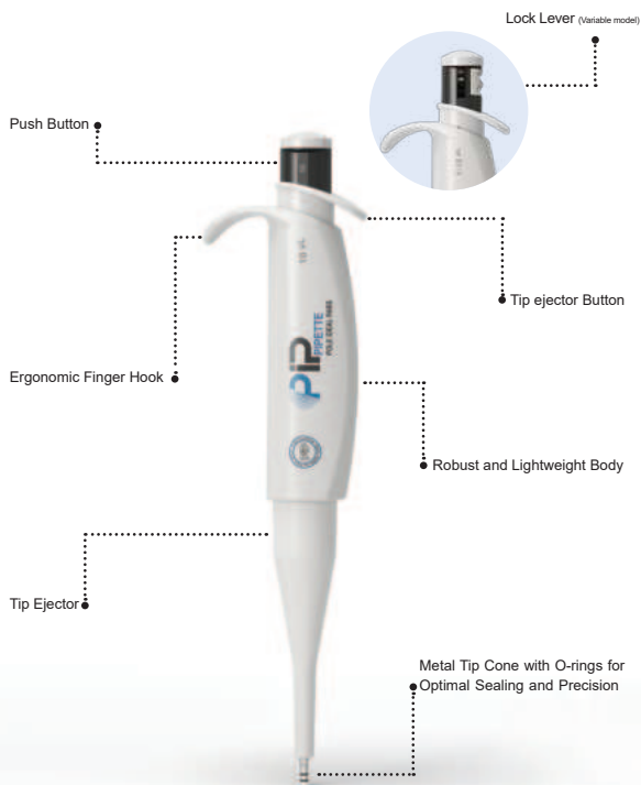
Figure 1. P.I.P. Pipette Overview
